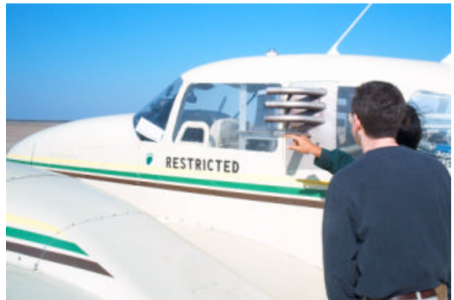
Figure 2. Air inlets on Baylor University's Piper Aztec atmospheric research aircraft.
